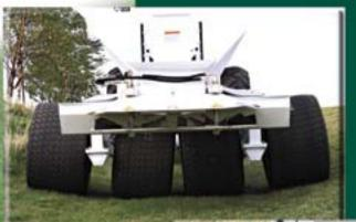
DAKOTA walking beam axles have the lightest footprint in the industry.
